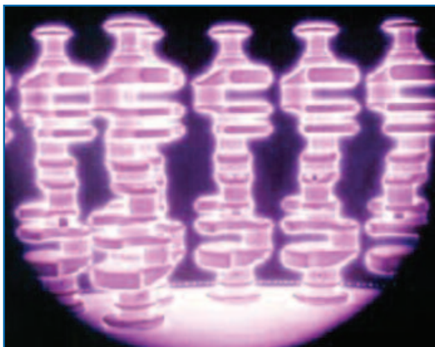
Ion Nitriding Shown - What you can see here is that the ENTIRE crank is getting treated evenly throughout.
