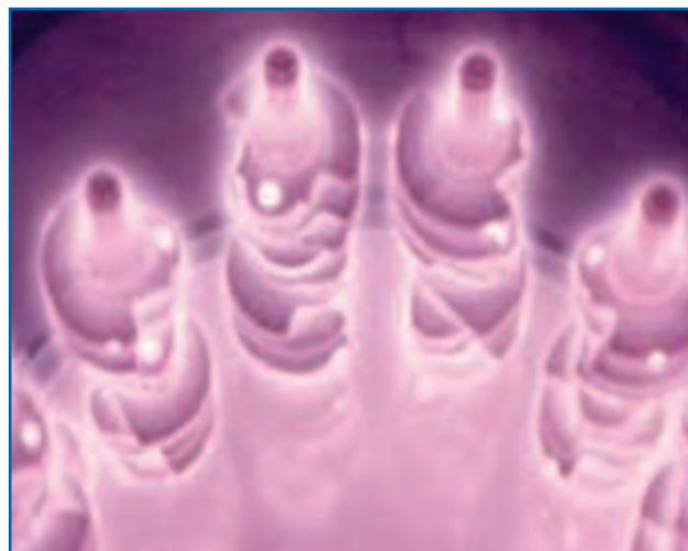
Ion Nitriding Shown - What you can see here is that the ENTIRE crank is getting treated evenly throughout.
